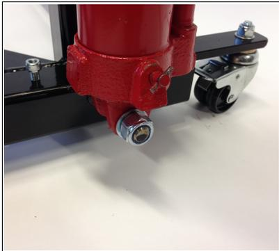
Fit the hydraulic pump by firstly locating it over the bottom pin and fitting the M16 nut and washer. Once you've tightened the nut, loosen it around 1/2 a turn to allow some free play in the pump on the bottom pin.
