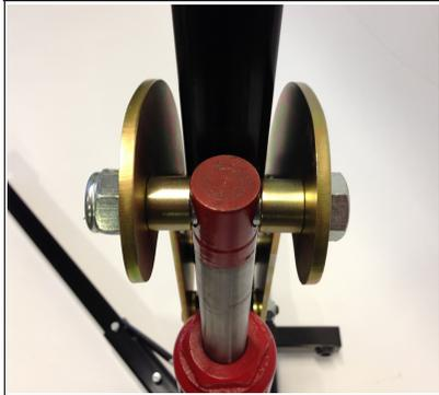
Pump the hydraulic pump up until the hole on top of the shaft is in line with the holes on the gold roller assembly. Fit the M16 nut and bolt using the 2 gold centralising spacers either side of the pump to keep the pump shaft central. Once again, when you have tightened the nut and bolt loosen it by around 1/2 a turn so there is some free play in the 2 centralising spacers.
