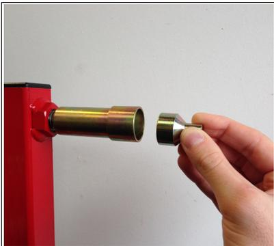
Finally if you have received a fitting kit for your bike with the Sky Lift check these are correct on either side of the swing-arm pivot on your bike and then insert them into the appropriate fittings each side of the Sky Lift.
