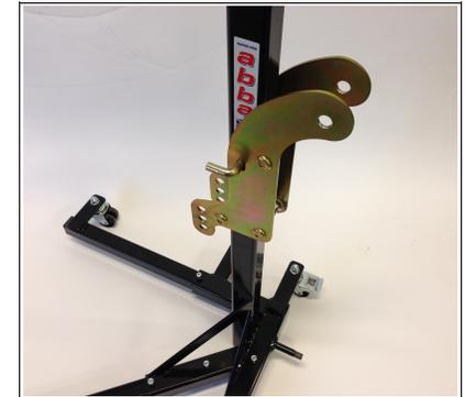
Next slide the gold roller assembly over the main upright of the lift and slide it down to the lower locking position. Line the holes up and slide through the locking pin so the roller assembly holds in place.
