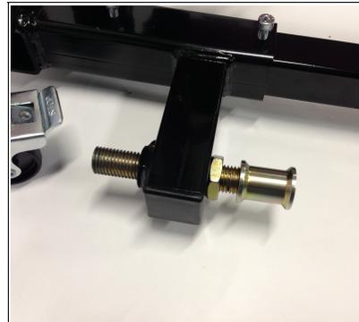
If you are intending to lift the bike in the wheelie position screw the strap mount into the black base of the stand.
