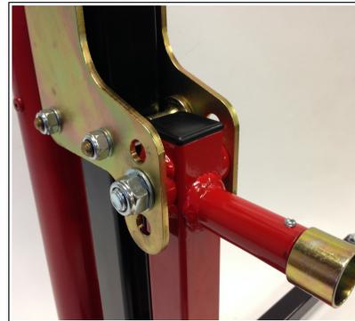
Slide the red section of the lift between the gold roller assembly plates and locate with the M14 nut & bolt. You'll notice there is 3 different height options, we recommend you start with the middle position. You can later change this up or down depending on the height of your swing-arm pivot. (ensure the bottom roller guides on the red section sit correctly onto the main upright)
