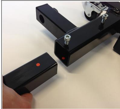
Firstly slide the three legs (black parts with wheels) into the three pockets on the main upright of the lift. Each leg has a coloured dot on it, slide the corresponding leg into each pocket. Two of the legs will slide in until they hit a stop.
