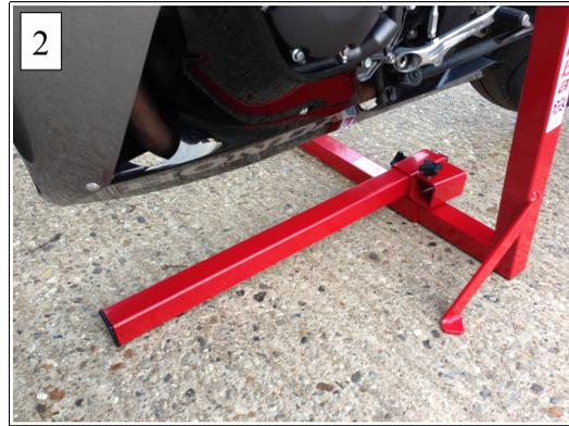
Once the superbike stand is fitted the tube should be free to slide along the base of the stand. Slide the tube along the base approximately a quarter of the way. This can be readjusted later.
