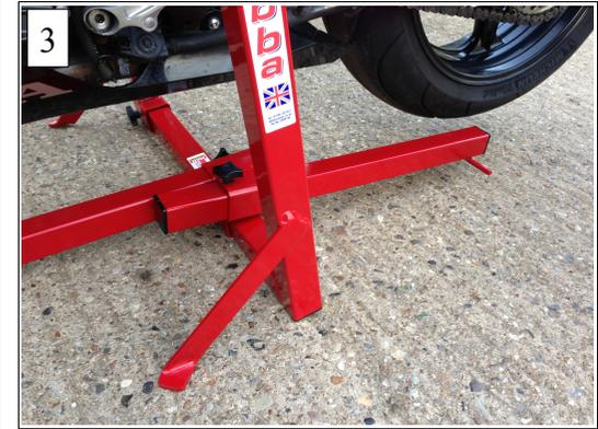
Next slide the second arm through the other tube with the pin facing outwards and horizontal to the ground. The arm is adjustable forward and back. Position the pin so that it is level with where you will attach the strap to the swing arm. Then tighten the thumb screw.
