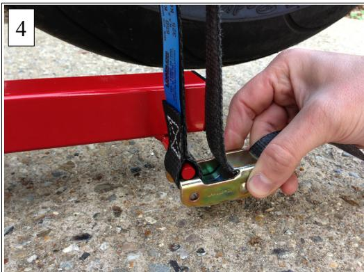
Feed the lifting strap around the swing arm and back through the buckle of the strap. If you have the optional bobbin pin feed the strap through the buckle first and place over the bobbin pin.
