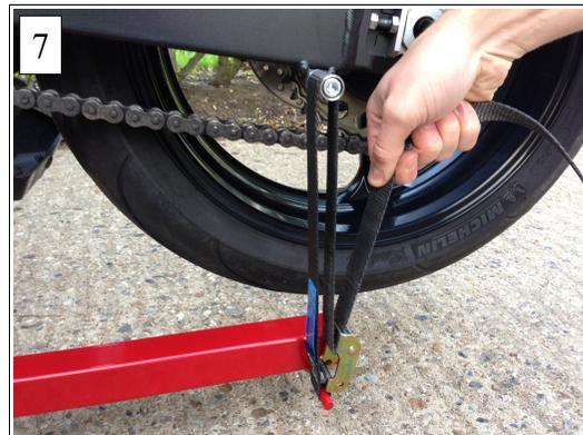
Finally by pushing down or leaning on the back of the bike while simultaneously pulling the lifting strap up the front of the machine should raise from the floor.
