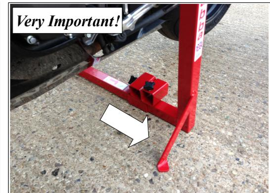
Before lowering the superbike stand, push the sliding tube up against the upright of the stand. Failure to do this could result in the tube section fouling the fairing/underside of the machine and damaging it.
