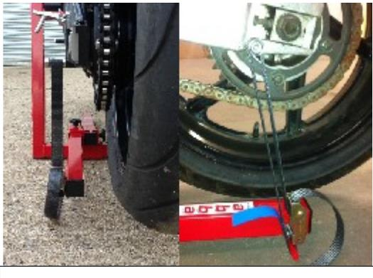
It is **very important** that when looking from the rear of the bike after the strap has been fitted the strap is perfectly vertical. This ensures the bike is pulled down straight when lifting. (As per left photo above)
